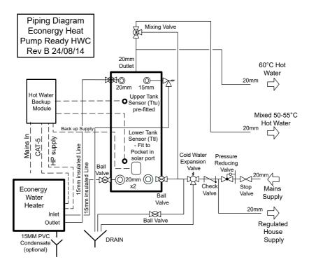
**Notes:** Piping Diagram 3: Connection to Econergy® Heat Pump Ready Hot Water Cylinder
