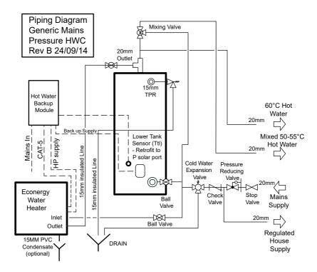
**Notes:** Piping Diagram 1: Generic Single Inlet Hot Water Cylinder Econergy Accessories Required:
