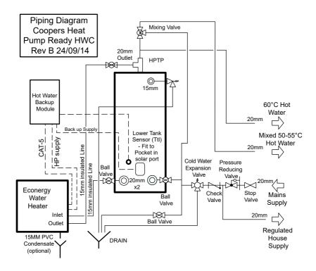
**Notes:** Piping Diagram 2: Coopers Mains Pressure Solar Ready Hot water cylinder
