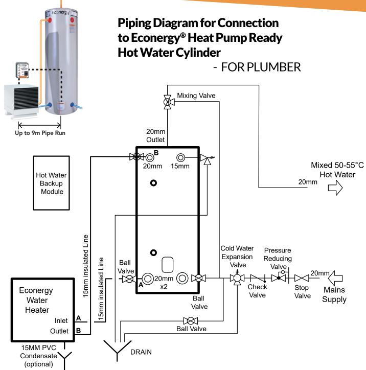
Please ensure inlet (A) is plumbed to the bottom of the cylinder (A) and outlet (B) is plumbed to the top of the cylinder (B).
